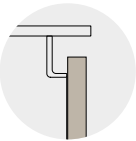
Gola con frontali dritti Groove profile with straight fronts
